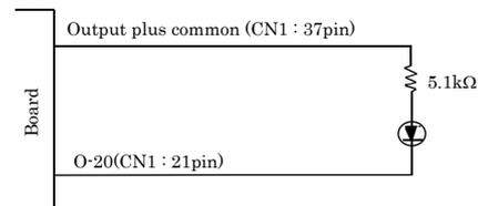
When "1" is output to a relevant bit, the corresponding LED comes on. When "0" is output to the bit, in contrast, the LED goes out.
