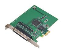
This product is a PCI Express bus-compliant interface board used to provide a digital output function on a PC.
