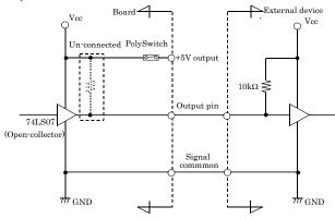
\* O-xx represents an output pin. One polyswitch is connected for Vcc(+5V) terminal.
