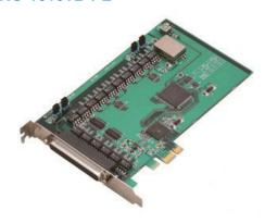
This product is a PCI Express board used to provide a digital signal I/O function on a PC. This product features TTL level input 16ch, TTL level output 16ch opto-coupler isolated type with an internal 5VDC power supply that does not require external power. You can use all of the input signals as interrupt inputs. In addition, digital filter function to prevent wrong recognition of input signals is provided. Windows/Linux driver is bundled with this product.
