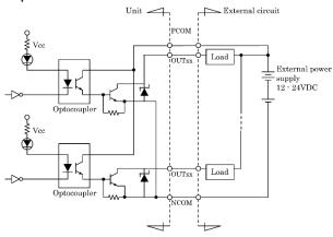
Figure shows the output circuit for the interface section of this product. The signal output section consists of an Optocoupler isolated open collector output (current sink type). An external power supply is therefore required to drive the output section of this product.
