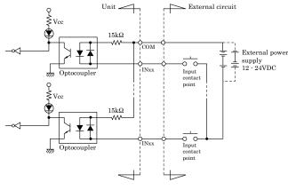
Figure shows the input equivalent circuit for the interface section of this product.
