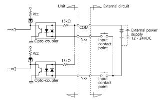
The signal input section consists of an Opto-coupler isolated input (compatible with both current sink output and current source output). An external power supply is therefore required to drive the input section of this product. The power requirement for this product is about 0.8 mA per input channel at 12VDC (about 1.6 mA at 24VDC).
