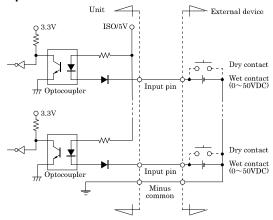
The input circuit of interface blocks of this product is illustrated in the above figure. Each input channel accepts either dry contact or 0 - 50 VDC wet contact inputs.
