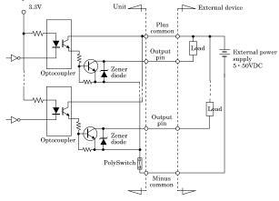
The output circuits of interface blocks of this product are illustrated in the above figure.
