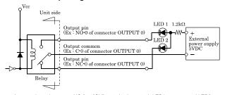
As a result, setting output NC-0 to "ON" state (make status), LED1 goes out and LED2 comes on.
