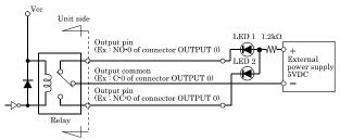
As a result, setting output NO-0 to "ON" state (make status), LED1 comes on and LED2 goes out.
