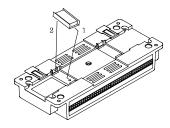
To remove the magnet, slide the magnet in the direction of arrow 1 as shown in the following figure, and then lift it out in the direction of arrow 2.
