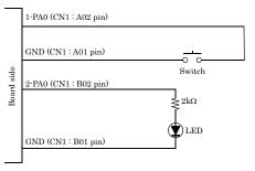
When switch is "ON", the corresponding bit is "0". When switch is "OFF" in contrast, the corresponding bit is "1".
