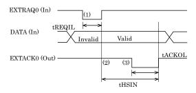
tREQIL: EXTREQO low width 50ns (Min.) tACKOL: EXTACKO low width 100ns tHSIN: Handshaking time 100ns (Min.)
