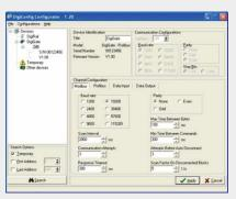
During the configuration process, the Modbus interface of the **DigiGate** will stop working as a master and start operating as a slave. On this condition, a computer equipped with a USB-RS485 is connected to the Modbus interface, and **DigiConfig** software will work as a Modbus network master in order to perform the **DigiGate** configuration.
