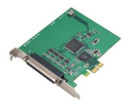
The < DI-32T-PE > features 32 unisolated TTL level inputs. You can use 32 input signals as interrupt inputs. In addition, the digital filter function to prevent wrong recognition of input signals is provided.
