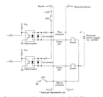
The input circuits of interface blocks of the DI-32B-PE are illustrated above. Connect the input signals to a device which can be current-driven, such as a switch or transistor output device.
