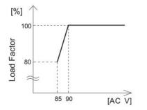
Input voltage derating curve
