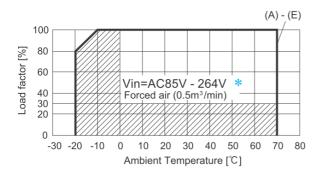
Derating curve depend on ambient temperature
