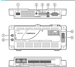
1 12 Name Function This is a connector for power. (Use the 3-pin connector included in the package) Power Connector 2 Debug Connector Do not use this.
