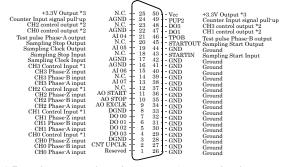
\*1 The control input can serve as the general-input, counter start/stop, preset, and zero-clear. \*2 The control output can serve as the general-output, count match, abnormal input error and digital filter error \*3 Supply-capable current is 500mA (Max).
