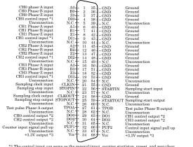
\*1 The control input can serve as the general-input, counter start/stop, preset, and zero-clear. \*2 The control output can serve as the general-output, count match, abnormal input error and digital filter error. \*3 Supply-capable current is SOMA (Max.).
