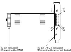
\* 37 pin D-SUB connector is the same as with the CN1.
