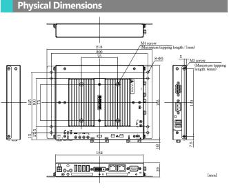
\*1 The length (L) from the tip of M4 boss to the M4 screw tip should be 5mm or less. If not doing so, it may be exactly fixed.
