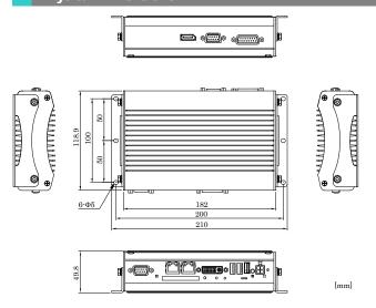
\*1 When you fasten the bundled attachment fittings to be fixed to the body, you should use the attached screws (M4 x 10). Otherwise, the length (L) from the surface of the cabinet to the screw tip should be 5mm or less.
