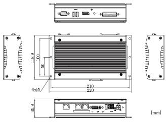
st When you fasten the bundled attachment fittings to be fixed to the body, you should use the attached screws (M4 x 10).
