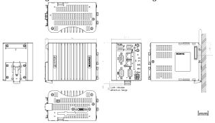
To secure this product with the included fittings, use the included screws (M3x7). In other situations, use screws with a penetration depth (L) from the chassis surface to the screw tip of 3 mm or lower.
