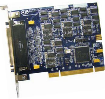
Fully PCI 2.3 compliant, the BlueStorm/SP can be installed in any 3.3V or 5V system.
