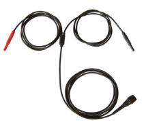
ence. With a conventional oscilloscope with standard oscilloscope probes this is not possible. The maximum distance between the positive side and ground of a standard oscilloscope probe is usually limited to approximately 20 cm. The Measure lead TP-C1812B for the Automotive scope ATS5004D does not have this limitation and allows you to measure between points that are more than 2 meters apart, without picking up external interferences.
