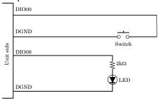
When switch is "ON", the corresponding bit is "0". When switch is "OFF" in contrast, the corresponding bit is "1". When "1" is output to a relevant bit, the corresponding LED comes on. When "0" is output to the bit, in contrast, the LED goes out.
