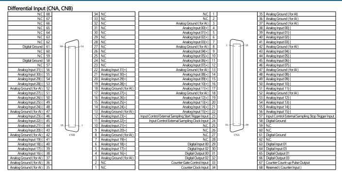
Pin Assignment of interface connector (Differential Input)
