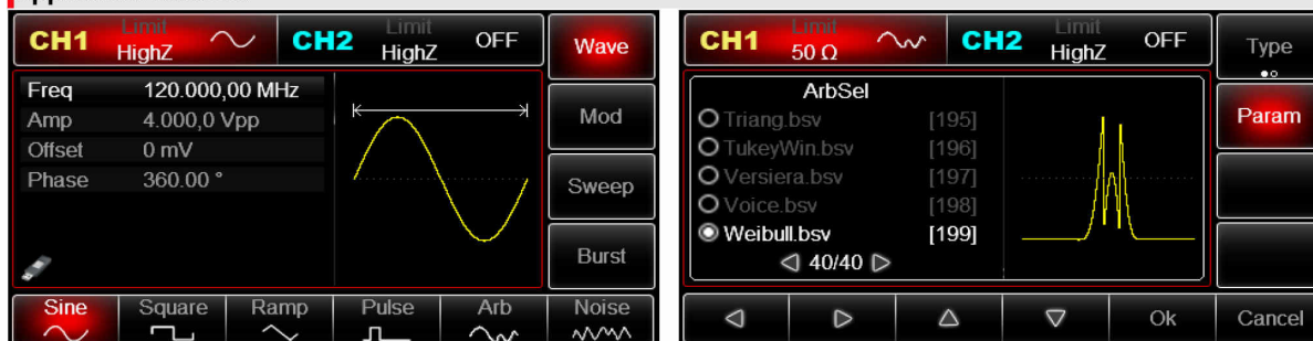
120MHz sine waveform output, Double Channel and Multiple Waveform Selection
