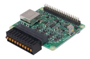
This product is an expansion card that adds an analog Input interface to the Raspberry Pi.
