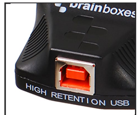
High retention USB connection requires a minimum withdrawal requirement of 15N (thats a force of 1.5Kg or 3.4lbs)
