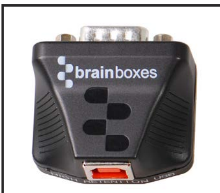
IP-50 rated non-conducting case
