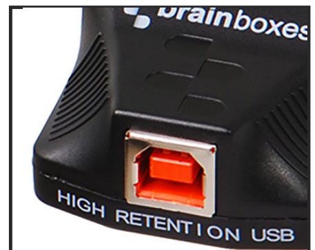
High retention USB connection requires a minimum withdrawal requirement of 15N (thats a force of 1.5Kg or 3.4lbs)
