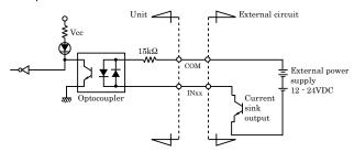
Example of a Connection between Input and Current Sink Output
