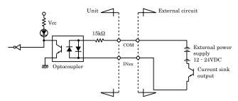
Example of a Connection between Input and Current Source Output
