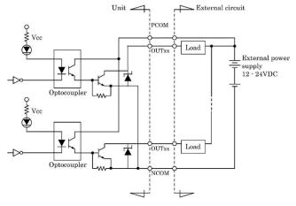
Figure above shows the output circuit for the interface section of this product.
