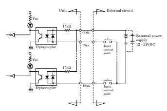
Figure above shows the input equivalent circuit for the interface section of this product.
