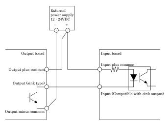
Example of a Connection between Output and Input
