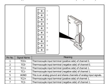
Thermocouple Input Cable
