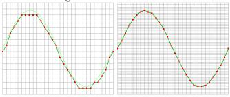
To display a signal measured with the Handyscope HS5 High Resolution oscilloscope at the same level of detail as the standalone oscilloscope, the display can be
