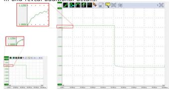
Shown are two displays, both showing a measurement of the same signal. The left display size corresponds to a size comparable to a standalone oscilloscope; at 8 bit resolution, zooming will not reveal more details. The right display corresponds to a maximized window on a standard PC screen; at 14 bit resolution, zooming will still reveal more details.
