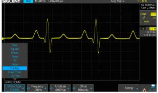
10 built-in waveforms plus 4 ARBs. The arbitrary waveforms can be accessed and edited by the EasyWave PC software
