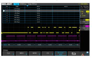
Displays the decoding through the events list. Bus protocol information can be quickly and intuitively displayed in table form
