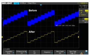
Eres mode can improve the SNR effectively, without the dependence on the periodicity of signal and stable triggering
