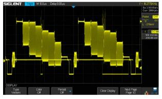
256-level intensity grading display on waveform
