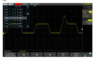
History function can record up to 80,000 frames of waveforms. The recording is executed automatically, so that the customer can play back the history waveforms at any time to observe unusual events, and locate the source quickly through the cursors or measurements. Located on the keyboard Panel, this function is easily accessible
