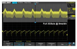
Using hardware-based Zoom technique and record length of up to 140Mpts, users are able to use a higher sampling rate to capture more of the signal, and then quickly zoom in to focus on the area of interest
