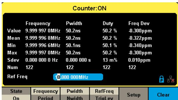
8-digit hardware frequency counter with statistics function and input range of 0.1 Hz ~ 400 MHz.
