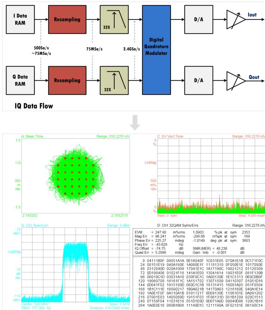
The SDG6000X supports popular modulation types such as ASK, FSK, PSK, and QAM. Proprietary resampling technology provides excellent EVM performance at arbitrary symbol rates between 250 Symb/s  $\sim$  37.5 MSymb/s. Built-in digital quadrature modulator provides the possibility to generate IQ signals from baseband to 500 MHz intermediate frequency.
