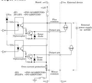
The output circuits of interface blocks of the PIO-16/16B(PCI)H and this product are illustrated the image above. The signal output section as an Optocoupler isolated open-collector output (current sink type). To drive the output section, the on-board internal power supply must be used or an external power supply is required.
