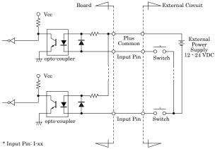
The input circuits of interface blocks of this product is illustrated in the image above.
