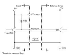
The input circuit of interface is illustrated in the image above. External digital signals given to signal inputs are TTL levels. The individual input signals are passed to the personal computer as active low signals. As each of the signal inputs is pulled up internally, the output of a relay contact or semiconductor switch can be connected directly between the signal input and the signal common pin.
