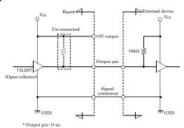
The output circuit of interface is illustrated in the image above. Signal outputs are open-collector outputs; individual output signals are sent to the external device as active low signals. Note that each signal output must be pulled up at the external device as it is not pulled up internally.
