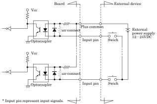
The input circuits of interface blocks of this product is illustrated in the bottom-left diagram. The signal inputs are isolated by opto-couplers (ready to accept current sinking output signals). The board therefore requires an external power supply to drive the inputs. The power requirement for each input pin is about 5.1 mA at 24 VDC (about 2.6 mA at 12 VDC).
