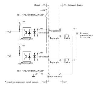
The input circuit of interface is illustrated in the image above. The circuit is connected to a device that can be current-driven, such as a switch or transistor output device.
