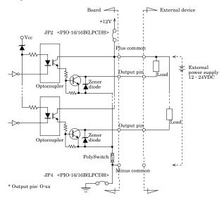
The output circuit of interface is illustrated in the image above. The signal output section is an opto-coupler isolated, open-collector output (current sink type).
