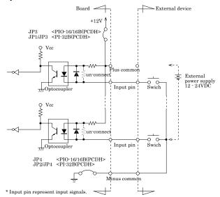
The input circuit of this board is illustrated in the image above. The signal inputs are isolated by the Optocoupler (ready to accept current sinking output signals). To drive the input section of the board, therefore, the on-board internal power supply must be used or an external power supply is required. The power requirement for each input pin is about 5.1 mA at 24 VDC (about 2.6 mA at 12 VDC).
