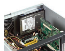
Shock-resistant drive bay for holding an internal 3.5" HDD
