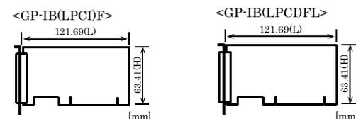
The standard outside dimension (L) is the distance from the end of the board to the outer surface of the slot cover.
