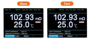
GOM-804/805 has two measurement speed selections, which are Fast reaching 60 readings per second, and Slow 10 readings per second. A major departure from the past, users, in the past, had to juggle between speed and display resolution. GOM-804/805 will not affect resolution despite of any speed selections and will maintain the highest display digits. In other words, reading resolution will not be changed by changing speed and the display digits remain the same.
