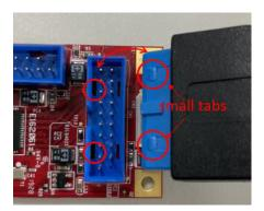
To pull off the USB 3.0 cable, DO NOT unplug the USB cable from the module directly, Wiggle Left- Right to release the small tabs from sockets then unplug the cable, refer to the below pictures for example:
