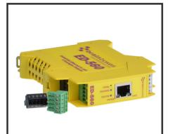
Non conducting polyamide casing with removable numbered terminal blocks for easy wiring
