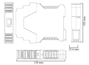
Screw Terminals 3.5mm pitch, #22 - #14, 0.5mm<sup>2</sup>-2.5mm<sup>2</sup> pin power supply
